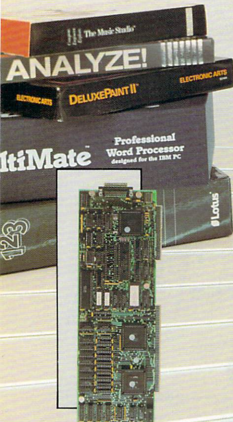
The Bridgeboard allows the Amiga 2000 to be IBM PC/XT-compatible.
